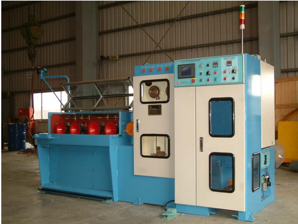
DC22/24 Fine wire drawing machine with Annealing system
